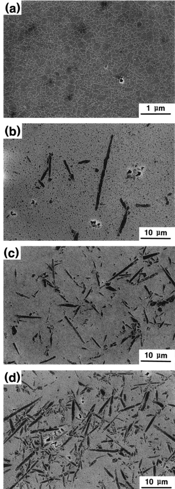
Figure 1 Typical microstructures of hot-pressed  $\beta$ -SiC ceramics containing (a) 0%, (b) 1 wt%, (c) 5 wt%, (d) 10 wt%, and (e) 20 wt%  $\beta$ -SiC whiskers as seeds.
