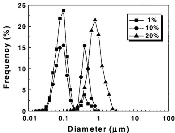
Figure 2 Grain diameter distribution revealed by the relation between grain diameter and areal frequency for 1 wt%, 10 wt%, and 20 wt% SiC whisker-seeded SiC ceramics.
