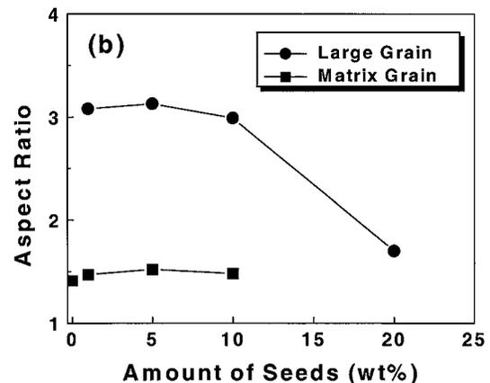
Figure 3 Change of (a) grain diameter and (b) aspect ratio of large grains and matrix grains for liquid-phase sintered  $\beta$ -SiC ceramics as a function of seeds content.
