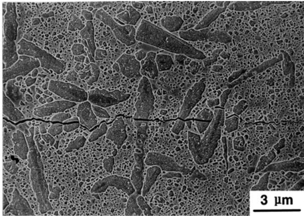
Figure 7 Scanning electron micrograph of a crack profile in the liquid-phase sintered  $\beta$ -SiC with 10 wt% seeds.
