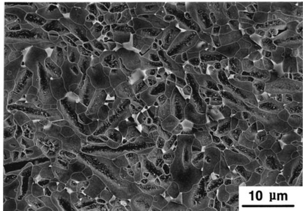
Figure 5 Typical microstructure of the hot-pressed and annealed  $\beta$ -SiC ceramics with 10 wt% seeds.
