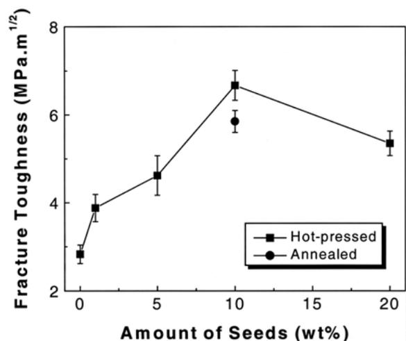
Figure 6 Fracture toughness of the liquid-phase sintered  $\beta$ -SiC ceramics as a function of seeds content.
